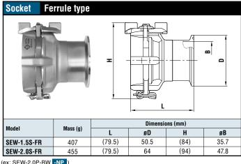
A type without seal material is also available. In such case, the model name ends with "-NP". (ex: SEW-2.0P-BW -NP
