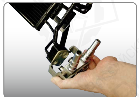
Helium Leak Test on Condensers
